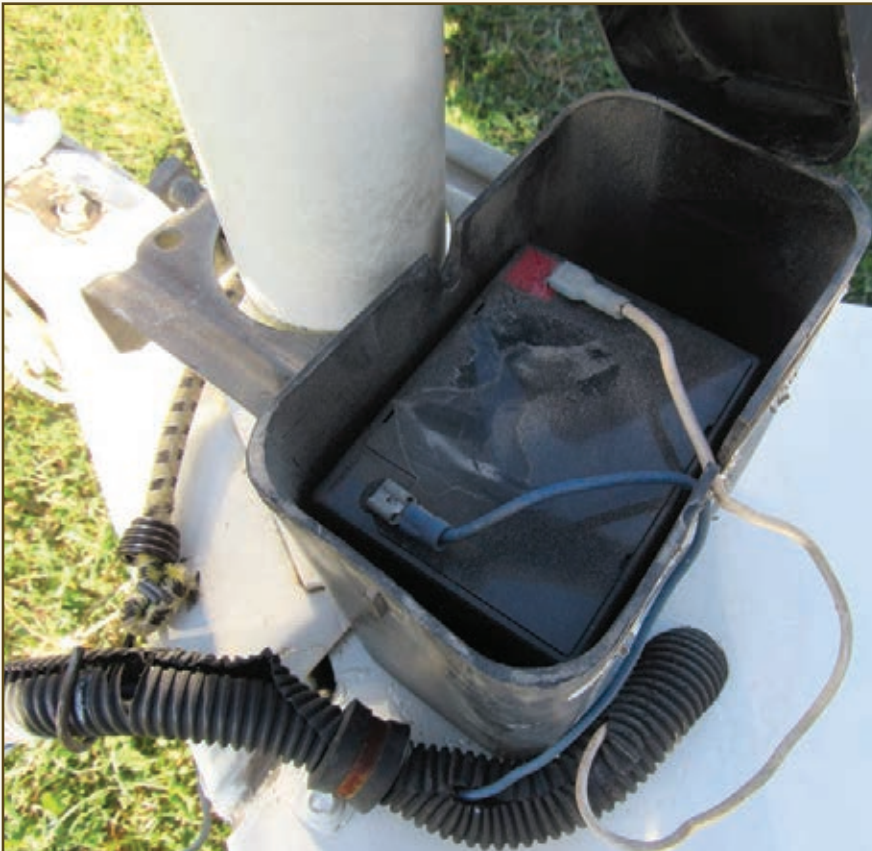
This breakaway brake system's battery is wired to be charged while the tow vehicle is running and is connected to the trailer.
