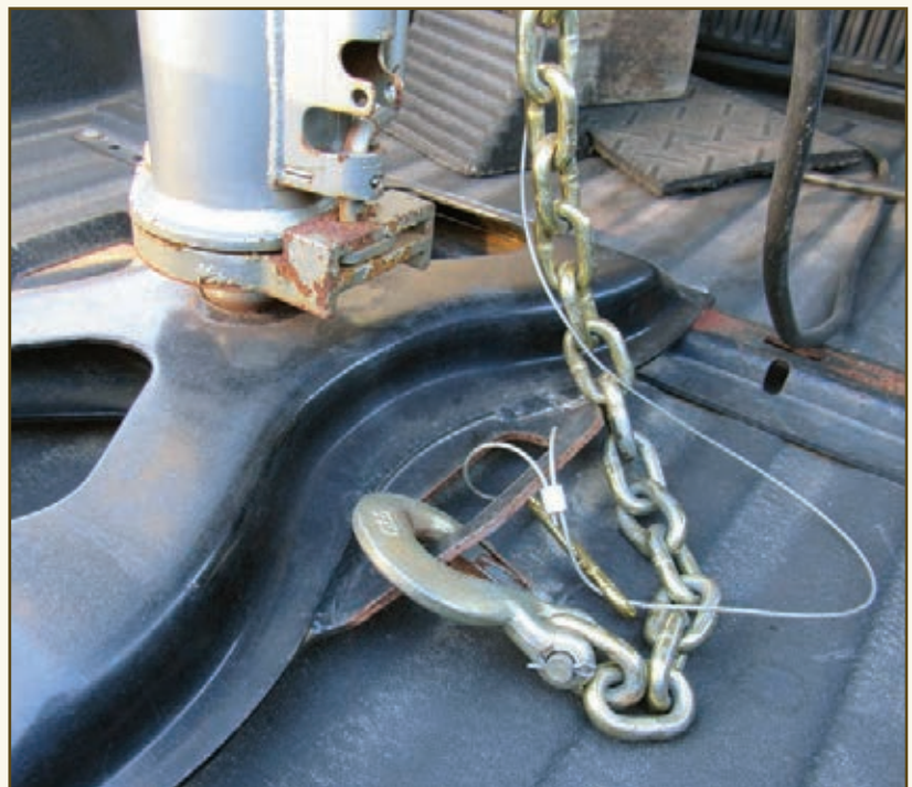
The cables for these breakaway brake systems are correctly hooked to the frame of the towing vehicle's receiver.
