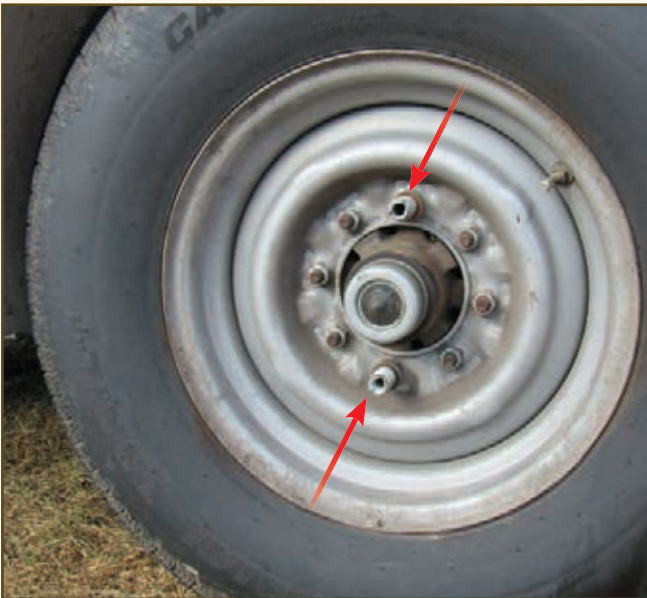
A special tool is required to take off the long pieces (arrows) that hold the cover to the wheel.
