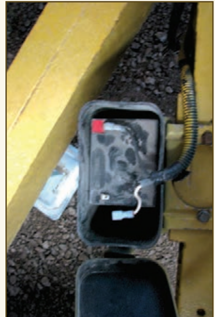
This brake system's battery has loose connections.
